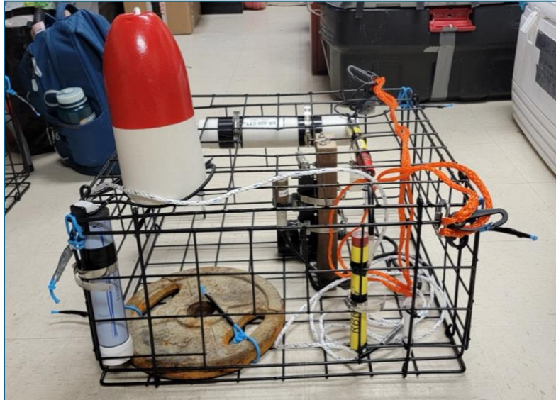
Figure 5. Mooring with cage design. Equipped with sensors to record temperature, pressure, salinity, turbidity and light. The moorings deployed in August were not equipped with a release mechanism for the buoy. These will have to be retrieved by diving in summer 2026.
