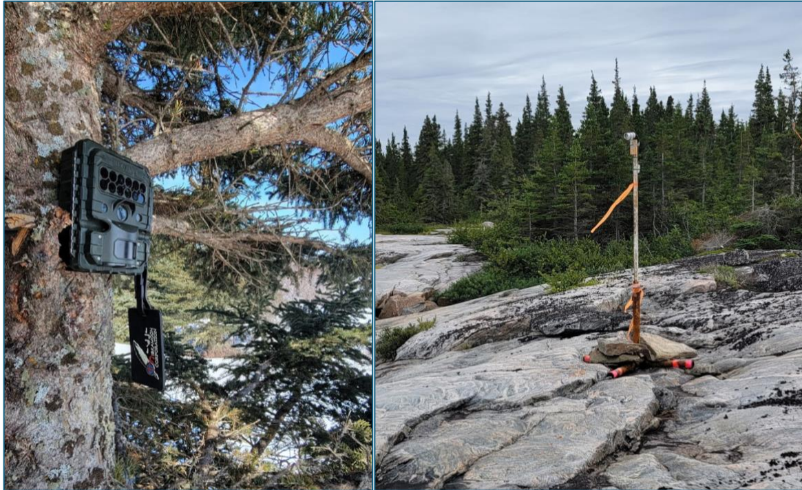
Figure 7. Examples of how cameras and IR sensors were set up along the coast. Cameras and IR sensors were pointed towards the coast to capture the water/ice around where the moorings are deployed.
